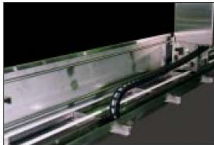
Cleanroom compatible belt drive and precision bearings.
